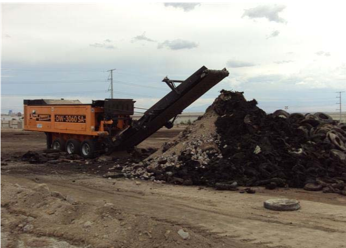
CAMU: Phase II, shredder sizing tires, etc.
