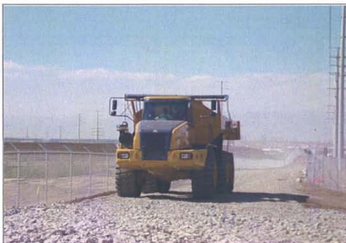
Westside: Haul truck on trackout rock proceeding to exit decon.
