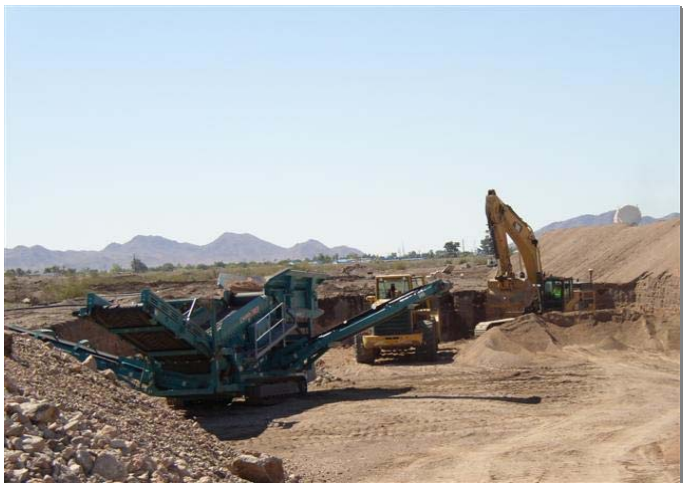
East side: Power screener processing 1 inch minus.
